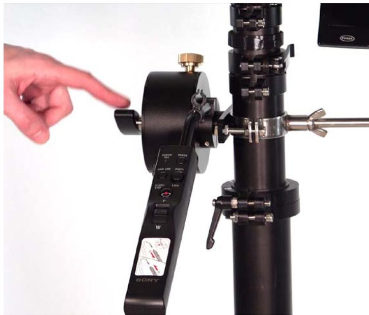
This handle has the black knob. It can be completely locked / open, or partially set to add custom drag to the motion.
