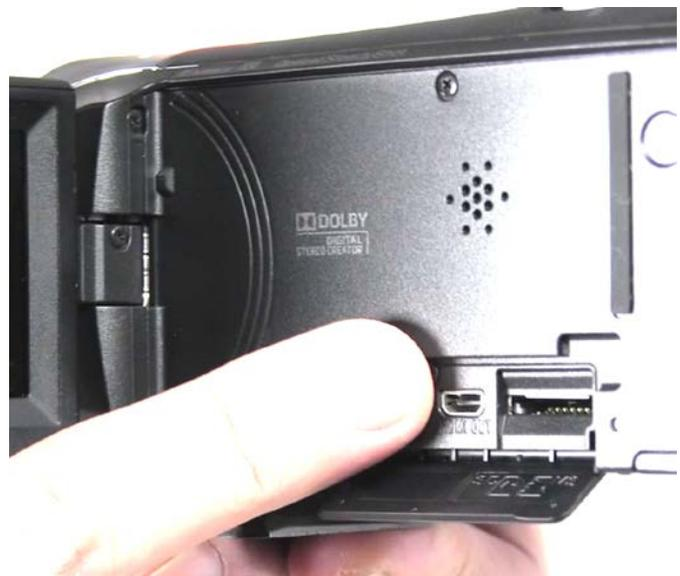
Regarding the SD port, once the SD card has been installed it's best to leave it in the permanently as the cards are very small. Inserting / removing the card over and over again is not advisable as you could cause damage. Instead, transfer footage out of the camera via the USB cable (to be discussed on the following page) located on the opposite side of the camera.
