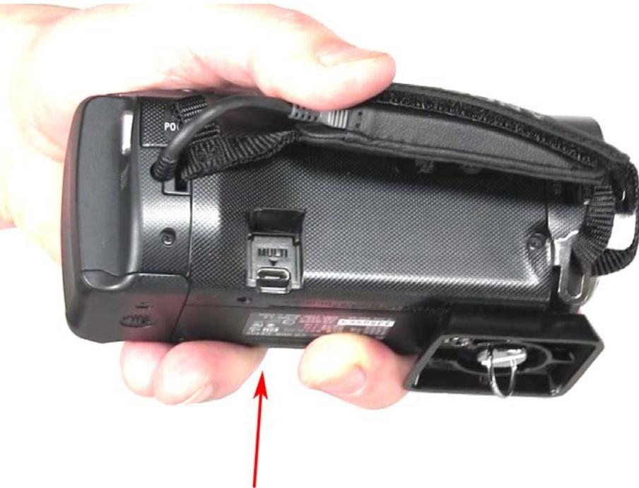
On the opposite side of the camera - under the hand strap - you'll find a small door. Open it and you'll reveal the 'Multi' port. This is where the cable will connect which sends signals to the camera from the remote control.
