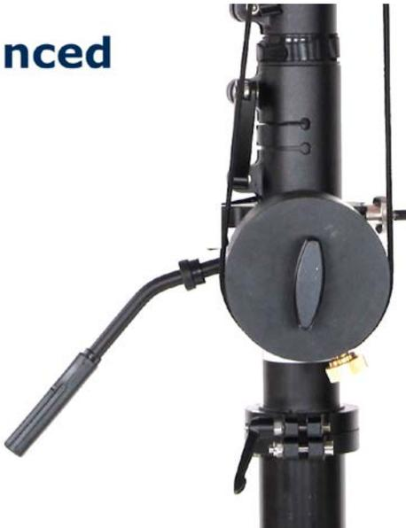
Note - each rope MUST go in opposite directions around the bottom of the handle. If this is not done correctly the handle will not be about to create the round motion which turns the head on top.
