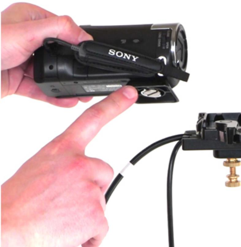
Notice how the camera already has a connection adapter attached to it. This is what you'll use to snap the camera to the quick release plate.
