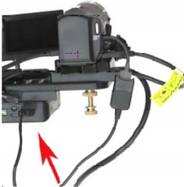
Then take the male end of the USB adapter and plug it into the USB power pack battery.
