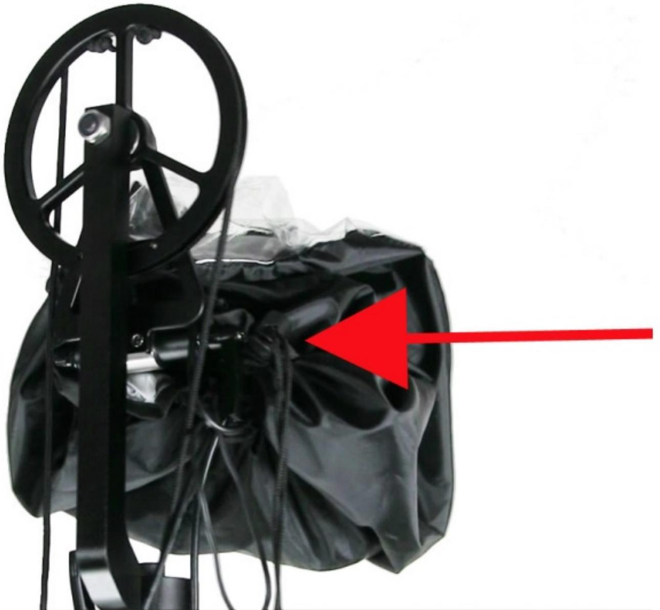
There is a cinch cord which will allow you to organize your cables, arrange the bag, and then completely close so no water can get inside. There are different ways to accomplish this, but the key is to pull the cord completely shut when finished.
