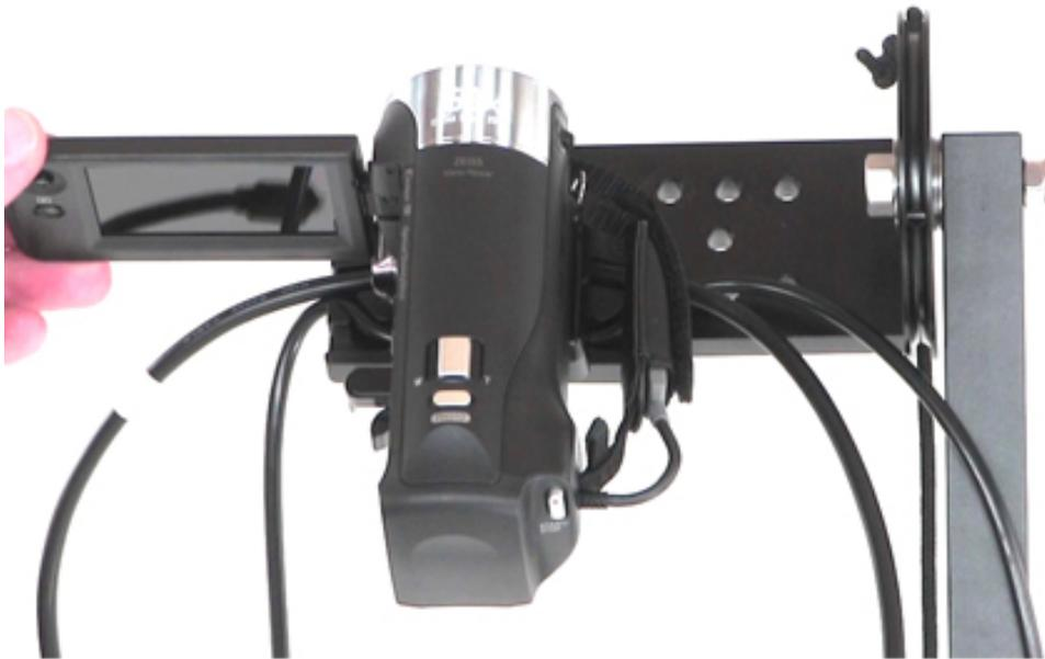
This image shows the camera snapped into the quick release plate. Pull back on the two levers on the quick release plate when it's time to pack up.
